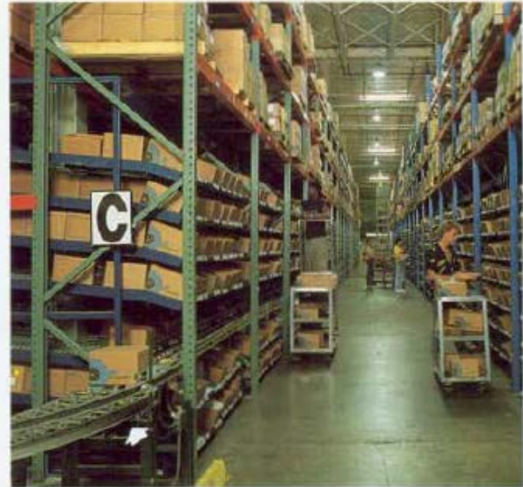
Keneco systems with crumpled shelves speed picking. System at right equipped with optional built-in takeaway conveyor (see arrow).
