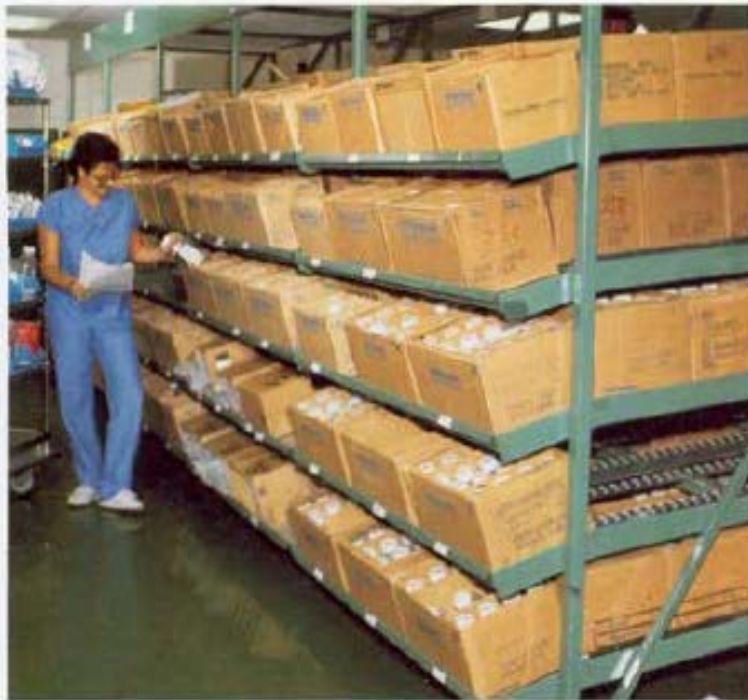
Keneco systems with crumpled shelves speed picking. System at right equipped with optional built-in takeaway conveyor (see arrow).
