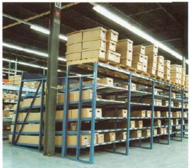
Restocking side of Keneco system. Single level pallet storage is provided above.
