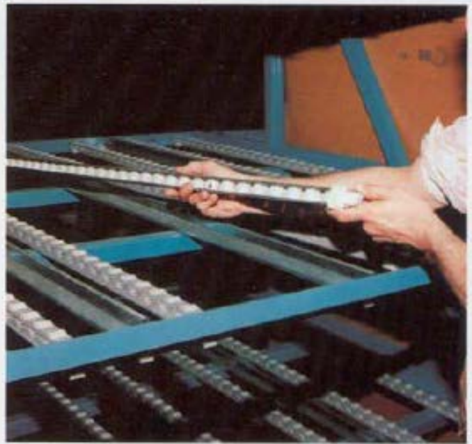
Kenrail track provides more wheels (on 1/8" centers) for better load distribution.
