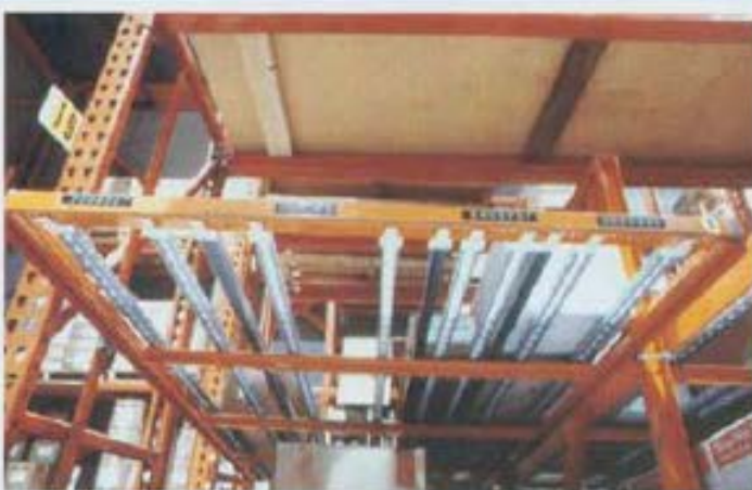
Shelf with gravity flow lanes is supported by pallet rack system. Keneco's ability to economically produce custom sizes which fit inside existing pallet racks results in material and space savings.
