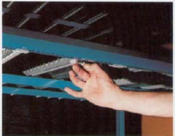
Special Keneco "klips" attached to ends of track speed installation and lane adjustment – without tools.
